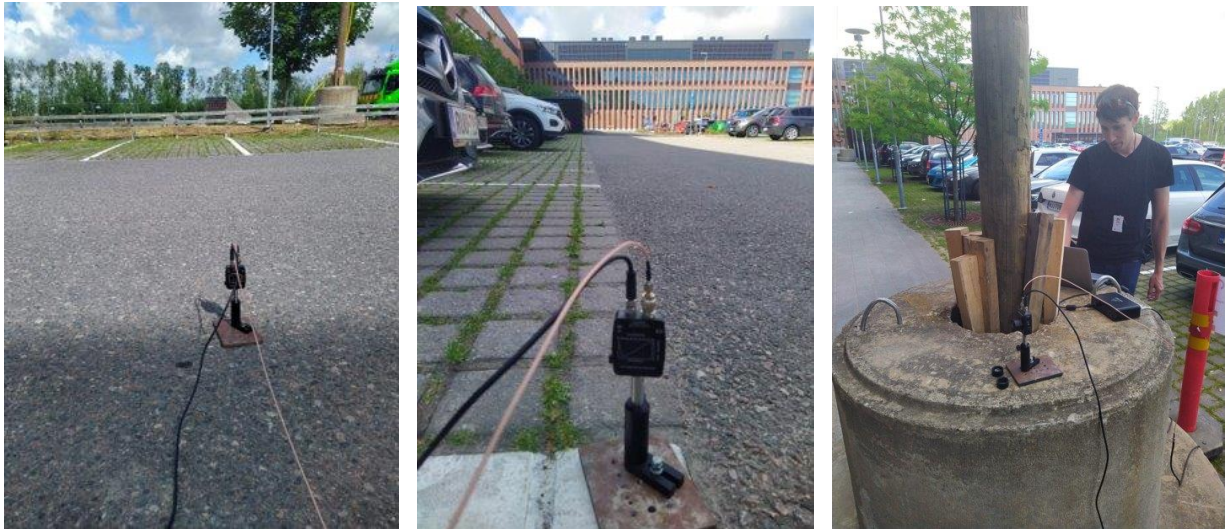
Figure 7. More pictures of the pilot preparation in the outdoor environment. All the components used here, including photodetector, pre-amplifiers and laptop computer are commercial off-the-shelf.
